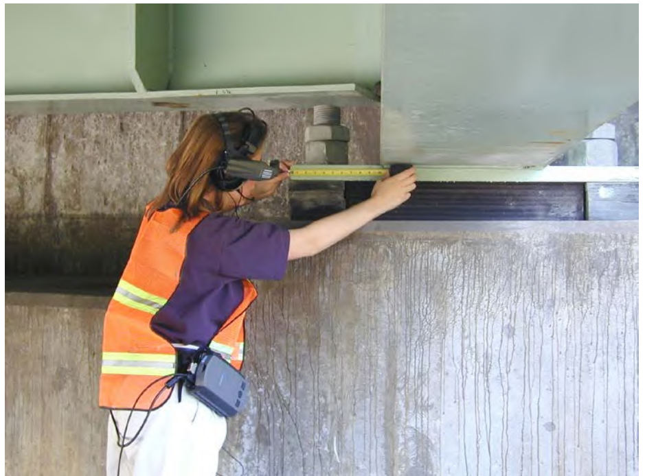
Figure 4.1.9 Inspector Using Wearable Computer
